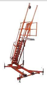
The Free-Standing Mobile Access Stair System (FSMASS) from Flexible Lifeline Systems® provides safe access for working surfaces up to 18'-3". The stair-step design provides safe access to and from work areas while carrying tools and each unit has two davit anchor points providing fall protection for two (2) users. Adjustable outriggers enlarge the base foot print to stabilize and level the system when in use and collapse into the base to create a small and mobile package for transportation.
